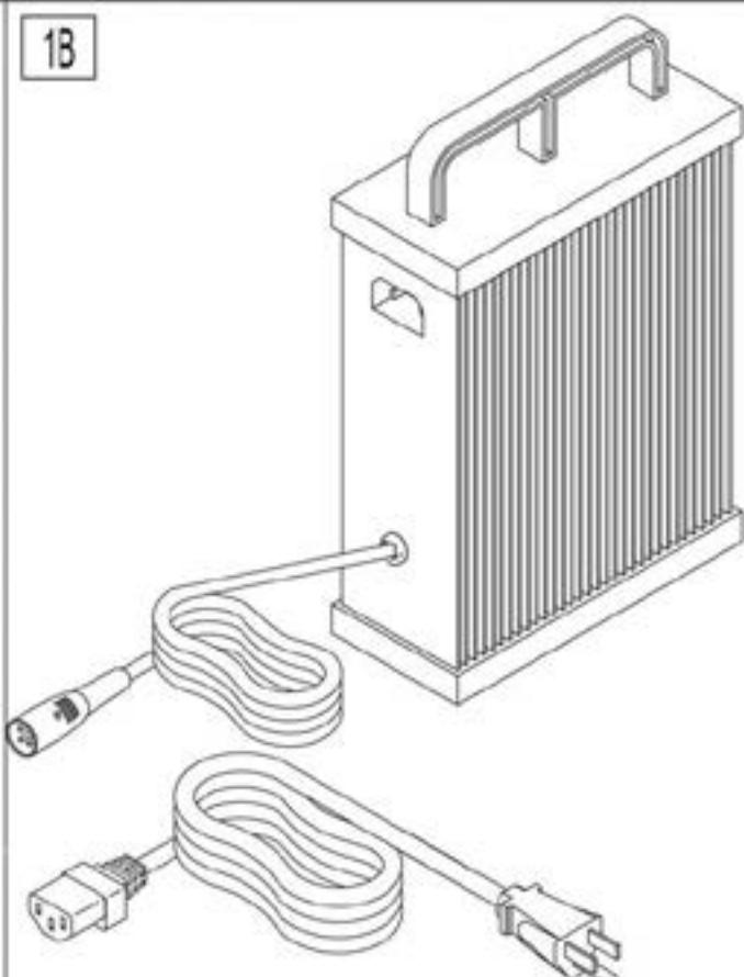
**WARNING:** Battery chargers are only intended to charge 24V, Group 22, Group 24, and Group 34 Lead Acid or Gel style batteries.
