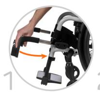
Insert the sub-frame into the docking clamps.
