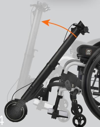
Push the handlebar forwards/ upwards until the locking bolt automatically clicks into place. Only release the wheelchair wheellocks once F35 is locked in place.
